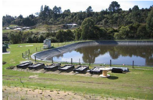
Figure: Trial of different denitrification beds at the Taupo District Council wastewater plant. Photo courtesy of GNS Science
